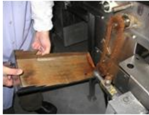
Fig 7. Example of material incompatible with cleaning solution / method
