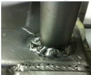
Fig 5. Poor sanitary welds are not cleanable at a microbiological level
