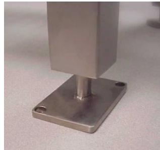
Fig. 14. Hermetically sealed hollow tubing
