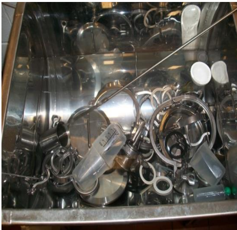
Fig. 18. Incorrect storage of parts in a COP tank. They should be stored in designated areas
