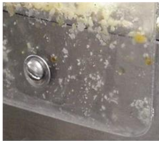
Fig 9. Splashguard requiring tool for disassembly and creating a catch point
