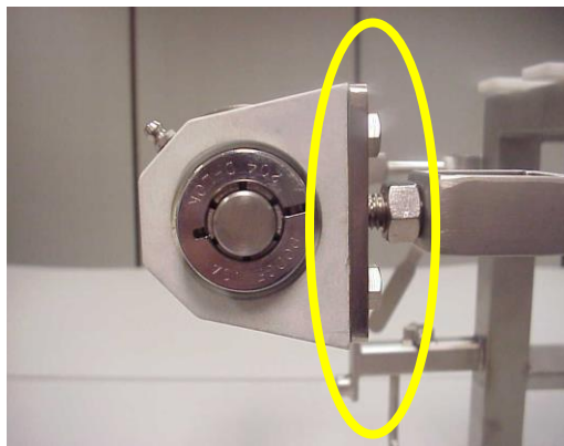
Fig. 23. Sandwich area formed by the bearing housing and framework where Listeria spp. had established a niche and the framework had rusted
